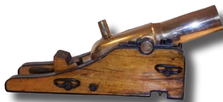
Lyle gun on display at Portland Head Lighthouse, Maine. USLHS archive photo.
